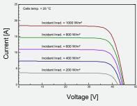
I-V CURVES OF PV MODULE(650W)
